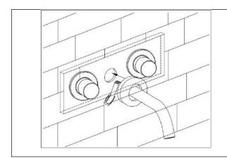
Apply sealing tape on the spout connector and fix it into the hole in wall, ensuring this is fully inserted.
