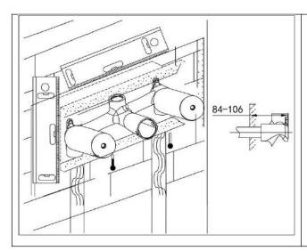
Based on the size of the body and the wall type, either secure it to the noggins or embed it into the wall at appropriate height and centre in relationship to the basin it will be servicing.
